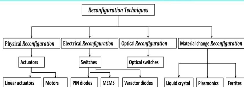
Fig. 4; Reconfiguration techniques of reconfigurable antennas.
