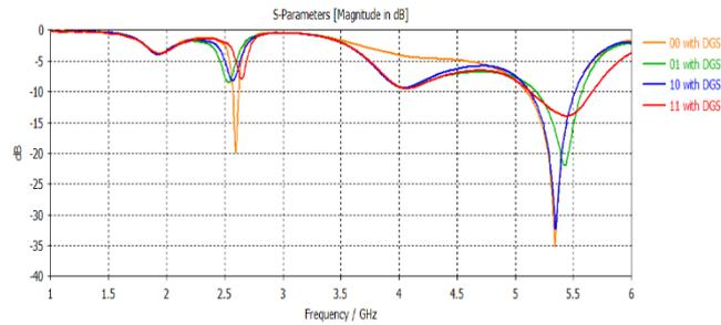
Fig. 6;  $S_{11}$  parameter of the proposal design.
