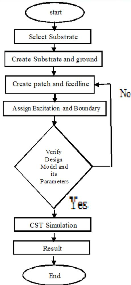
Fig. 2; The antenna simulation flow chart in CST.
